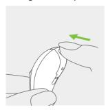
The battery is only tamperproof when the battery door is closed correctly. Always check after closing, that the battery door cannot be opened by hand.
